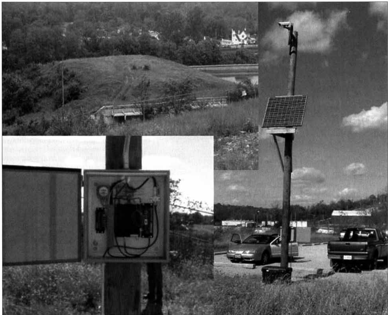
Fig. 2. Machine vision system monitoring the waste repository cap.
