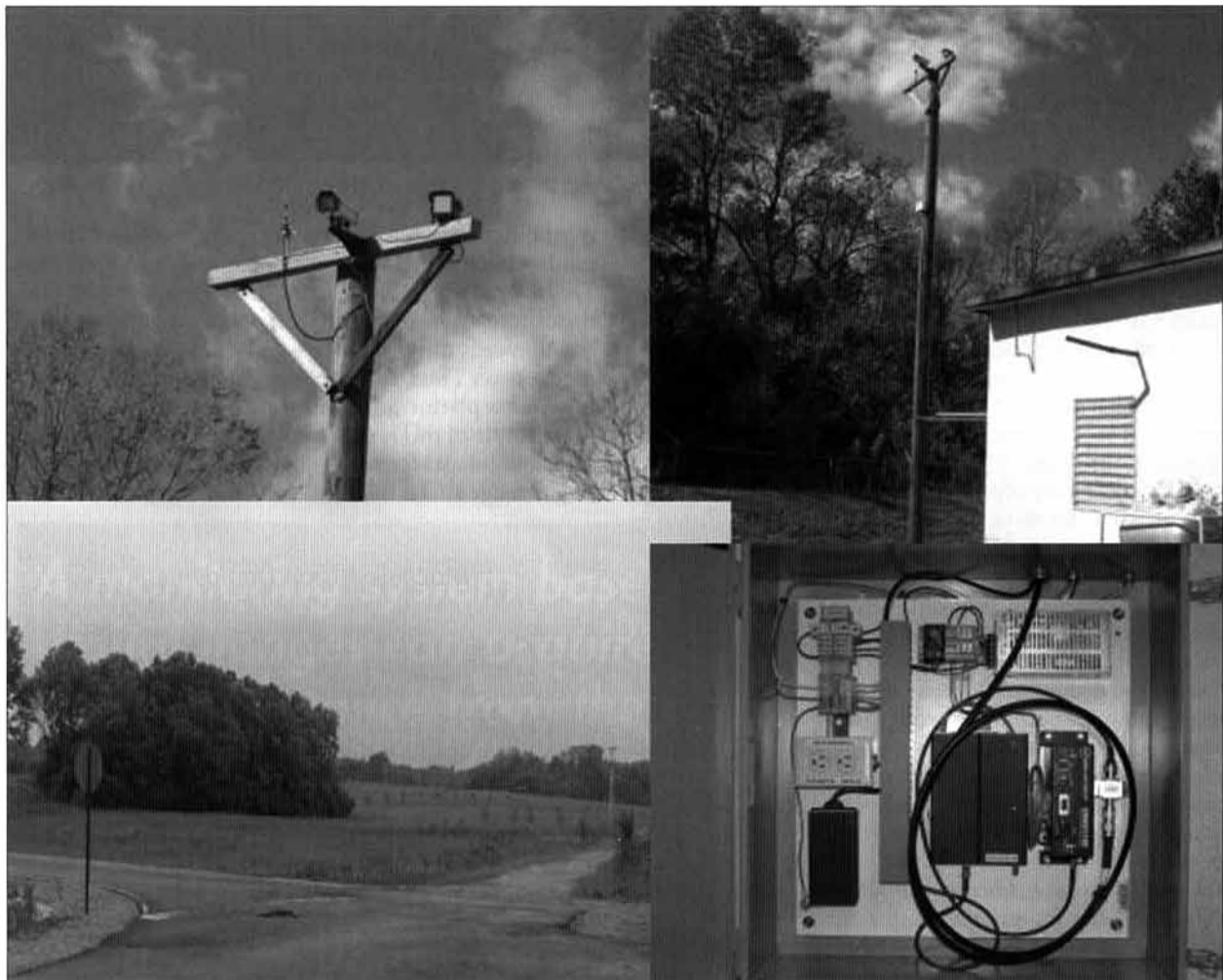
Fig. 3. The machine vision system with infrared illuminator monitoring for soil removal.
