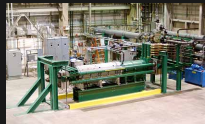
MSE Engineered, developed, constructed, and is testing an Ultrahigh-Pressure Test unit and facility to test and evaluate hypersonic-related materials, components, and systems to design and develop a successful mid-scale hypersonic wind tunnel.
