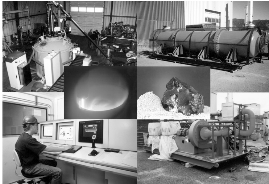
Clockwise from top left: 1) primary chamber/feeder skid; 2) secondary combustion chamber; 3) NO x skid; and 4) control room. Center left: plasma arc torch; center right: resultant slag.
