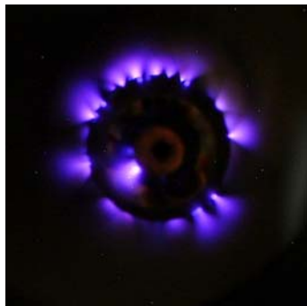
Figure 1. Corona discharge of 1-scfm test cell.
